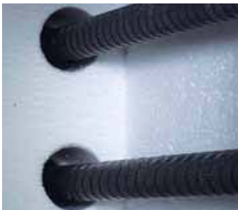
Furnace chamber with high-quality fibre materials and SiC heating rods on both sides of the furnace
