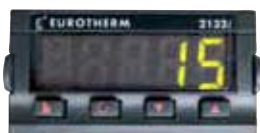
Over-temperature limit controller
