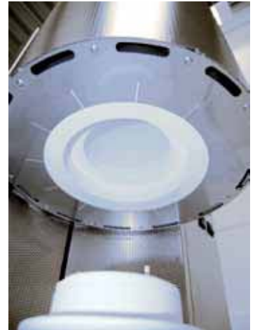
Plasma ceramic retort for protection of the heating elements and to avoid charge contamination in the LHT 02/16 LBR
